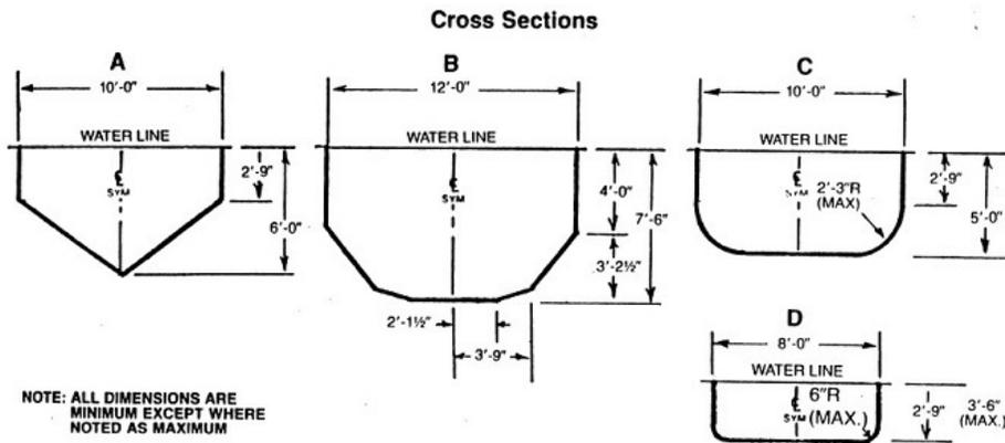
SECTION R326.10.10. This section contains Figure R326.10(6), minimum dimensions for a Type II pool.
