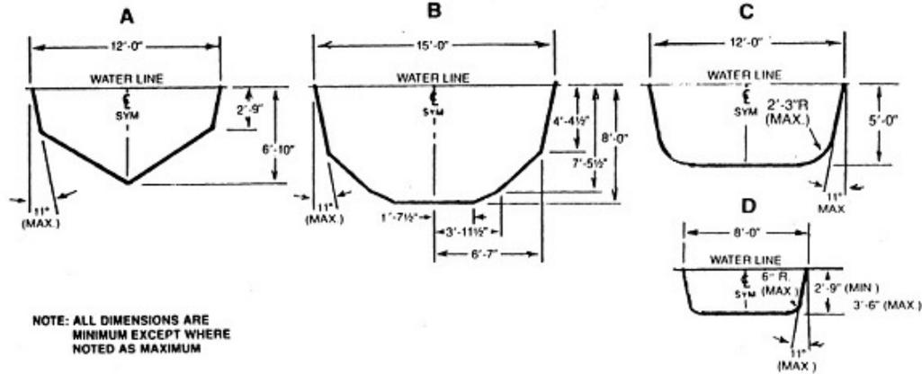
SECTION R326.10.12. This section contains Figure R326.10(8), minimum dimensions for a Type IV pool.
