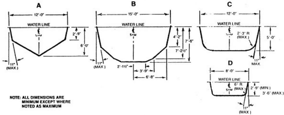
SECTION R326.10.11. This section contains Figure R326.10(7), minimum dimensions for a Type III pool.
