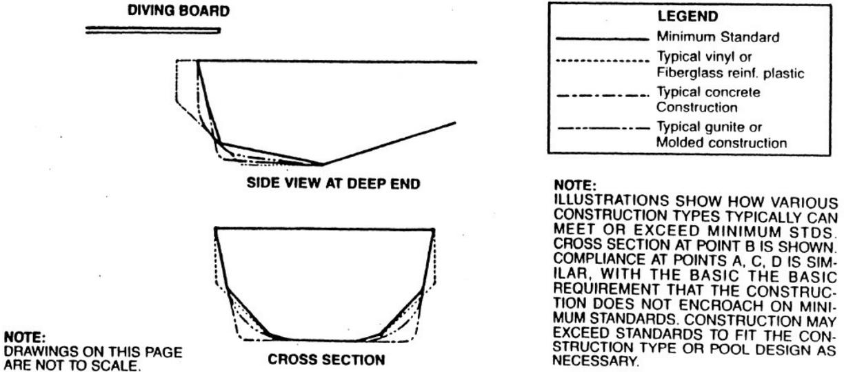
SECTION R326.10.9. This section contains Figure R326.10(5), minimum dimensions for a Type I pool.
