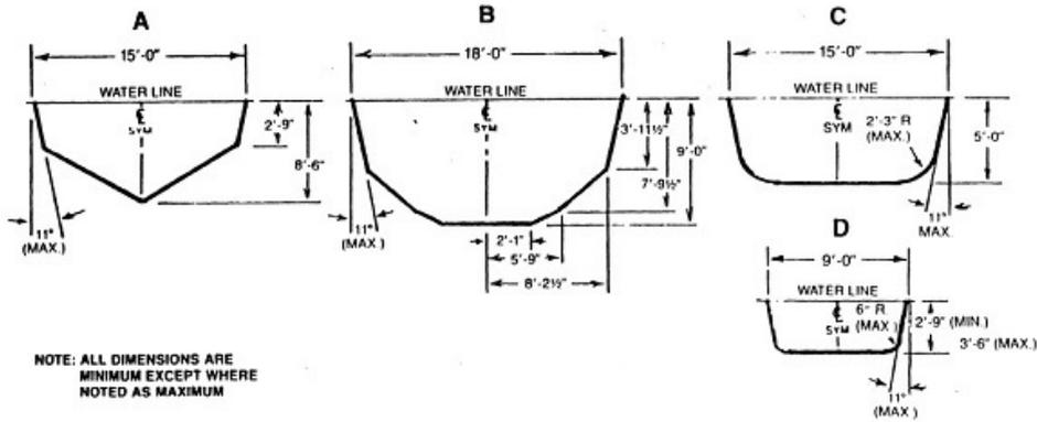
SECTION R326.10.14. This section contains Figure R326.10(10), shallow end detail for pool Types II through V.
