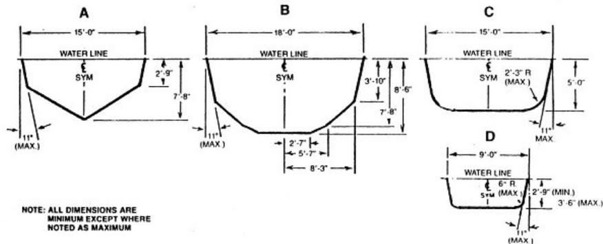
SECTION R326.10.13. This section contains Figure R326.10(9), minimum dimensions for a Type V pool.
