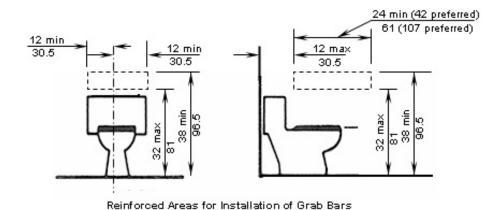
Figure 3 Water Closets in Adaptable Bathrooms
