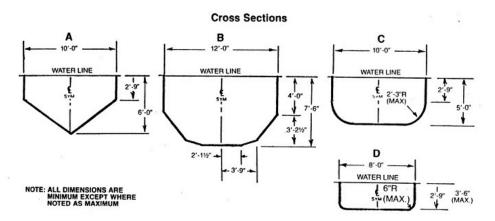
SECTION R326.10.10. This section contains Figure R326.10(6), minimum dimensions for a Type II pool. FIGURE R326.10(6)
