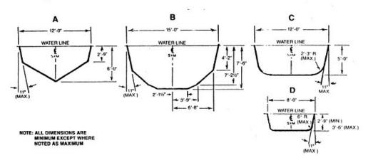
SECTION R326.10.11. This section contains Figure R326.10(7), minimum dimensions for a Type III pool. FIGURE R326.10(7)
