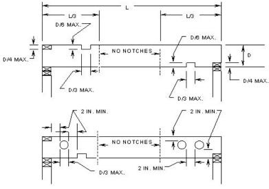
SOLID LUMBER JOISTS, RAFTERS AND BEAMS
