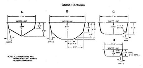
SECTION R326.10.13. This section contains Figure R326.10(9), minimum dimensions for a Type V pool.
