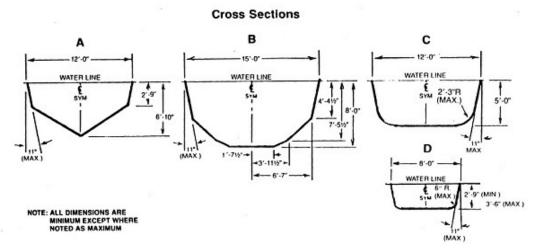
SECTION R326.10.12. This section contains Figure R326.10(8), minimum dimensions for a Type IV pool.
