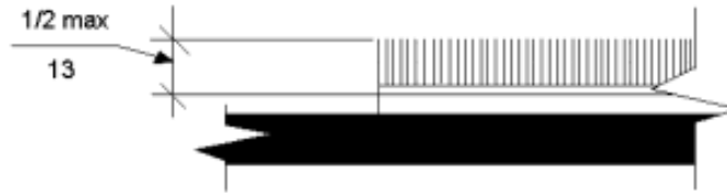
Fig. 302.2 Carpet on Floor Surfaces
