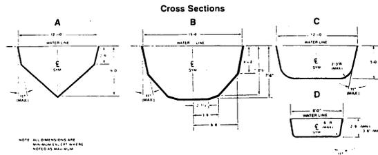
(f) This subsection contains Figure No. 4-7, minimum dimensions for a Type III pool.
