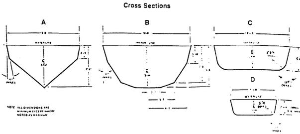
(h) This subsection contains Figure No. 4-9, minimum dimensions for a Type V pool.
