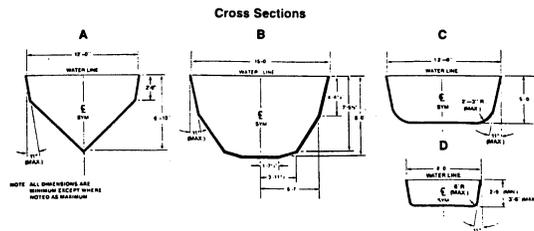
(g) This subsection contains Figure No. 4-8, minimum dimensions for a Type IV pool.
